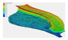
Fig. 2: Mesh of Lake Vernex model and the proposed canal (z amplified 8x)
